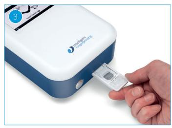
The Cartridge is placed in the Intelligent Fingerprinting DSR-Plus for analysis.
